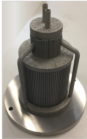
Figure 3 Heat exchanger produced by advanced manufacturing process – material IN617
