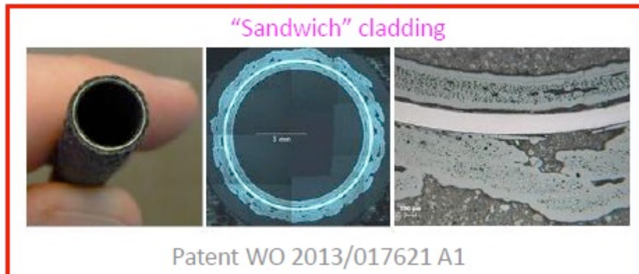
Figure 1 SiCf/SiC cladding – sandwich developed by CEA
