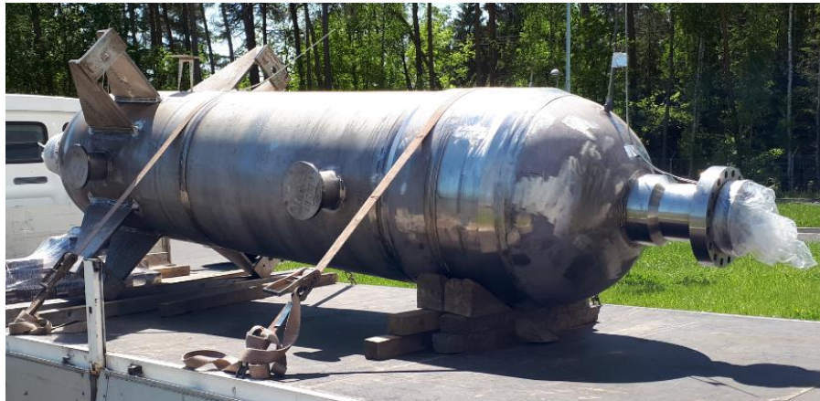
Figure 2-2: Primary heat exchanger of S-Allegro facility (transportation)
